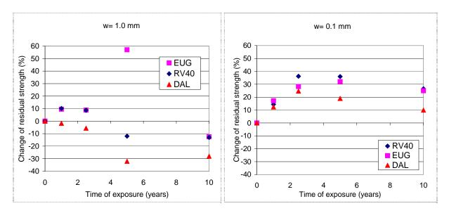
Figure 5: Development of residual strength for samples from mix WA30. Influence of exposure site, w= 1.0 mm (left), w= 0.1 mm (right)
