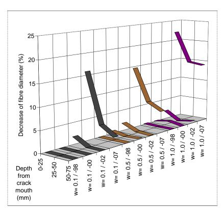
Figure 14: Decrease of fibre diameter for samples at at different time of exposure. Eugenia tunnel, Crack widths, Mix= WA30.
