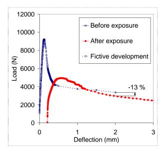
Figure 8: Change of residual strength - statistical approach. Development of residual strength at 2 mm deflection for samples from mix WA30.
