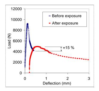
Figure 4: Change of residual strength - direct approach (w= 0.1 mm)
