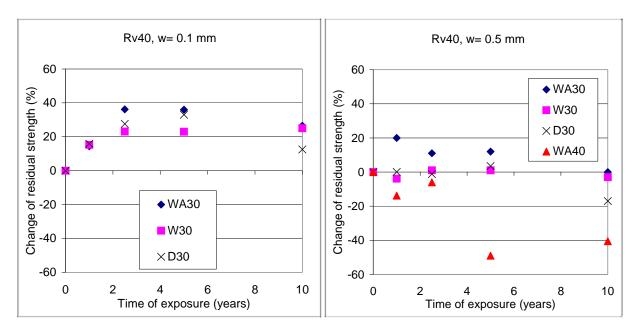
Figure 6: Development of residual strength for all types of mix. Rv40, w= 0.1 mm (left), w= 0.5 mm (right)
