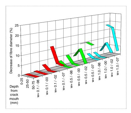
Figure 13: Decrease of fibre diameter for samples at different time of exposure. Rv40, Crack widths, Mix= WA30.
