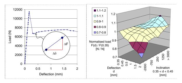
Figure 7: Definition of the inclination in the interval 0.35 < d < 0.45 (left). Average load development up to d=2 mm due to inclination (right).
