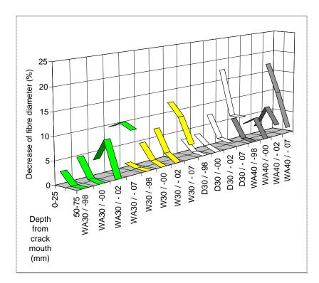
Figure 15: Decrease of fibre diameter for samples at Rv40 at different time of exposure. Mix types, Crack width w= 0.5 mm.
