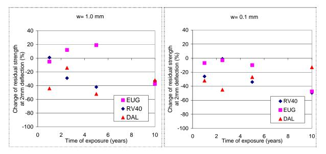
Figure 9: Development of residual strength at 2 mm deflection for samples from mix WA30. w= 1.0 mm (left), w= 0.1 mm (right). (Comparison with fictive values!)
