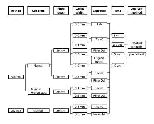
Figure 1: Field exposure test program
