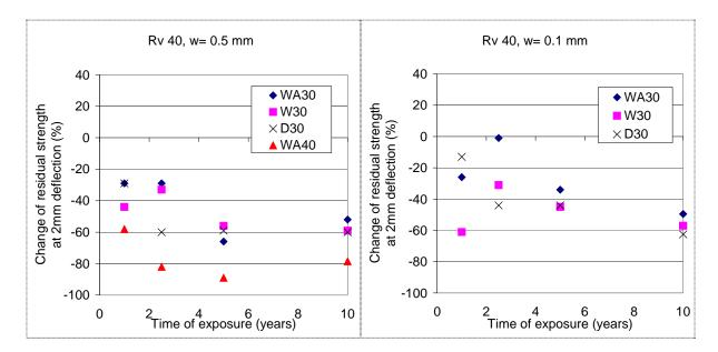
Figure 10: Development of residual strength at 2 mm deflection for all mix types. Rv40, w= 0.5 mm (left), w= 0.1 mm (right). (Comparison with fictive values!)
