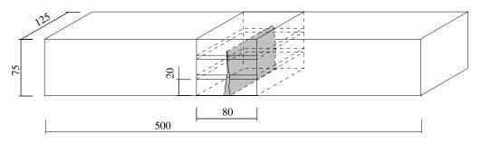
Figure 2: Dismembering of beams (measurements in mm)
