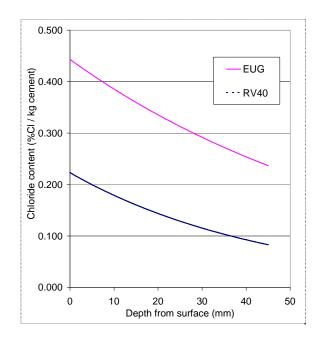
Figure 12: Average chloride profile from homogenous samples after 10 years of exposure. Exposure sites: Eugenia and RV40.
