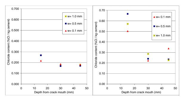
Figure 11: Chloride content at crack surface for WA30-samples after 10 years of exposure. Crack widths. Rv40 (left). Eugenia tunnel (right).
